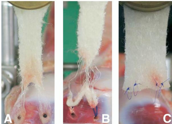
**FIGURE 4.** Typical examples of the failure mode of the tested fixation techniques: (A) failure mode of the pin fixation technique, (B) failure mode of the transosseous fixation technique, and (C) failure mode of conventional suture fixation technique.
