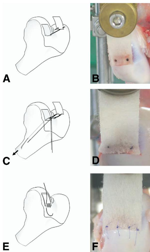
**FIGURE 1.** Schematic drawing and pictures of the fixation techniques tested. Pin fixation (A, schematic drawing; B, picture), transosseous suture fixation technique (C, schematic drawing; D, picture), and conventional suture technique (E, schematic drawing; F, picture).
