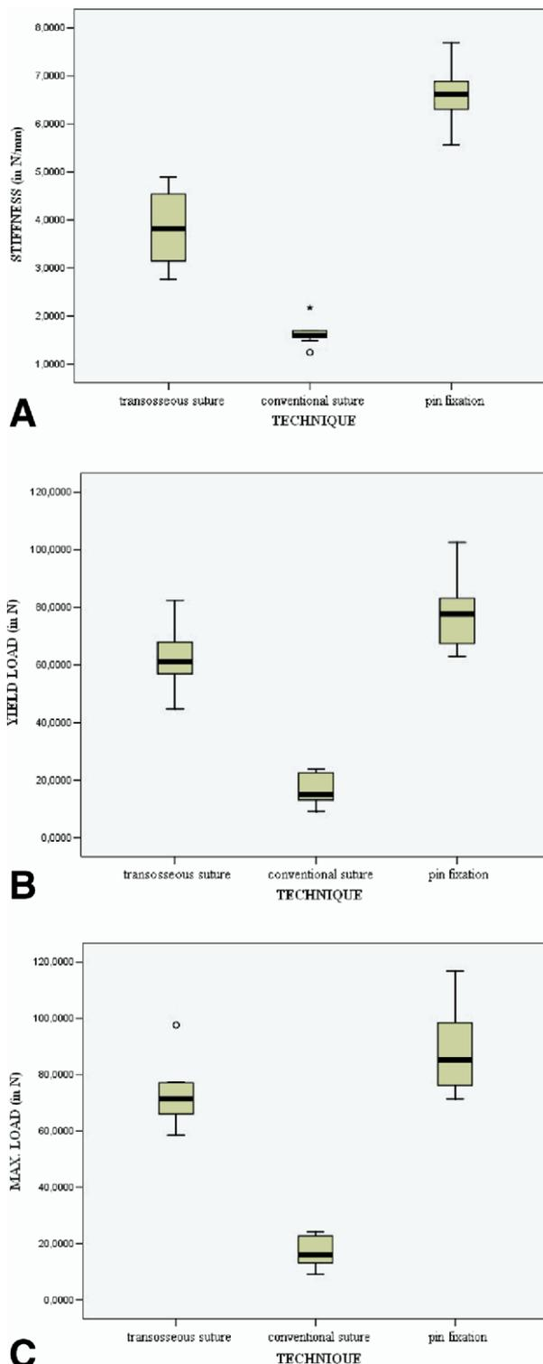
**FIGURE 3.** Box plots of structural properties: Stiffness (A), yield load (B), and ultimate failure load (C) of both arthroscopic fixation techniques are statistically significantly higher compared to the open conventional suture technique ( $P < .001$ ).
